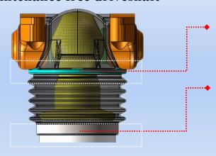
The two ends of the protective sleeve are fixed to the outer circle of the shaft tube and the outer circle of the nylon ball socket by clamps, forming a "static seal", so that the grease can never escape.
