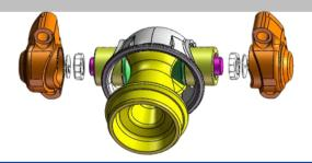
The universal joint of this product adopts the original "slotted pin shaft", "roller sleeve" and "ball joint" design scheme. This structure makes the transmission mechanism and direction change mechanism of the propeller shaft always in a closed lubrication space composed of rubber protective sleeve and nylon ball socket, so as to achieve the effect of maintenance-free, noise reduction and shock absorption.
