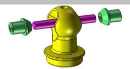
The slotted pin shaft is subjected to a balanced tension force in opposite directions at both ends when working, and has a stronger bearing capacity than a cross shaft of the same diameter. The whole shaft adopts the airfoil structure design scheme, if the main engine connection is simply modified, the connection flange between the two ends of the drive shaft and the upper and lower power ends can be simplified, and two flanges will be saved.
