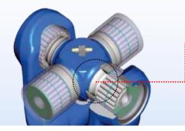
The "sliding seal" formed between the bearing seal and the cross-shaft journal causes grease to continue to escape during operation.
