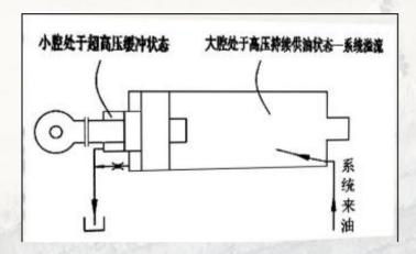
The oil inlet chamber continuously supplies high-pressure oil until the system overflows
